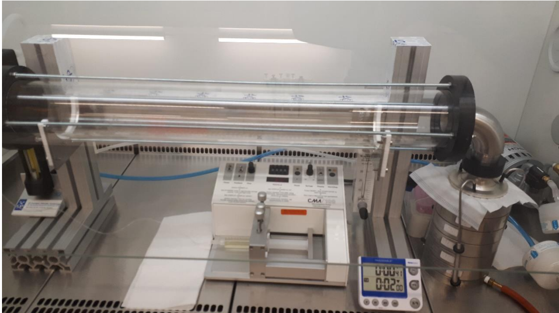
Figure A1: Set-up with test item mounted in the impactor.
